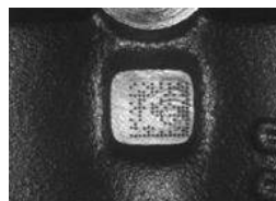
Dot Peening On Scratched Surface
